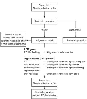
More stringent adjustment requirements: Ensure that the device is correctly aligned in the near range of 0.2 m ... 0.6 m. Object detection after successful Teach-in:
