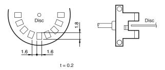
$\begin{tabular}{ll} \textbf{Response frequency}\\ \textbf{The response frequency is the value when the disc is rotated, see figure.} \end{tabular}$
