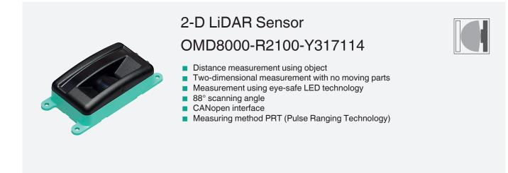
Multi-ray LED scanner for measuring the distance to an object, measuring method: PRT, measuring range: up to 8 m on white, 2x M12 plugs
