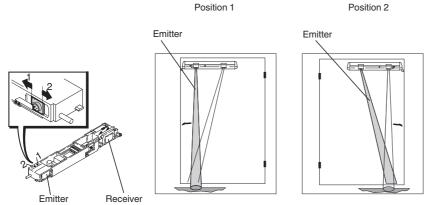
The transmitter of each sensor features two beam position settings via which the monitoring edge can be aligned to the left or to the right.
