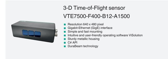
The 3-D time-of-flight sensor is based on the principle of measuring time-of-flight of infrared light. This allows raw 3-D data from objects at a range of 400 to 7500 mm to be acquired with an image resolution of 0.3 MP and a frame rate of 30 fps. The sensor features a Gigabit Ethernet interface, intuitive operating software, rugged metal housing, and an API interface. The sensor is especially suitable for dynamic applications with a larger measuring range.
