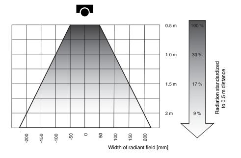
Radiant field Radiation < 50 % standardized to center axis
