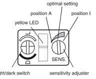
For optimal setting, now turn the sensitivity adjuster to the middle position between the positions A and B.
