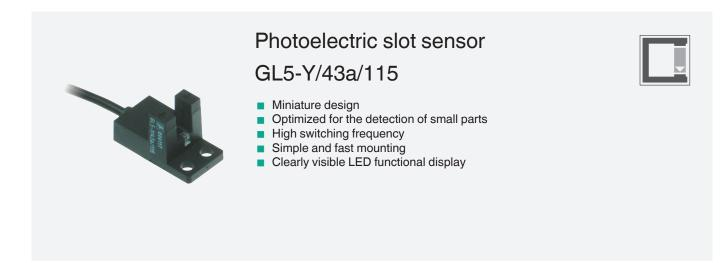
Miniature photoelectric slot sensor for the detection of small parts, Y design, fork width 5 mm, infrared light, PNP outputs, fixed cable
