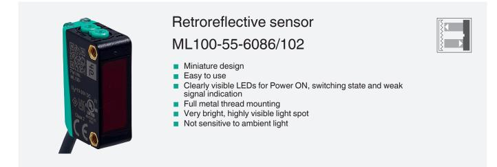
Retroreflective sensor with polarization filter, plastic housing, 5 m detection range, red light, sensitivity adjuster, light/dark on, DC version, NPN output, fixed cable
