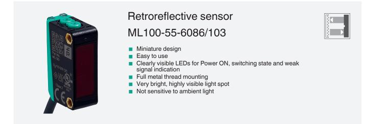
Retroreflective sensor with polarization filter, plastic housing, 5 m detection range, red light, sensitivity adjuster, light/dark on, DC version, PNP output, fixed cable
