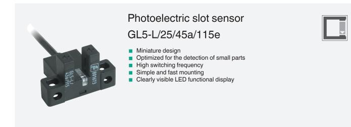
Miniature slot sensor for small part detection, L design, 5 mm slot width, infrared light, NPN output, light on, 150 mm fixed cable with JST plug, 3-pin
