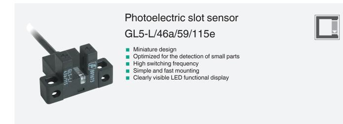
Miniature slot sensor for small part detection, L design, 5 mm slot width, infrared light, PNP output, dark on, 150 mm fixed cable with JST plug, 3-pin
