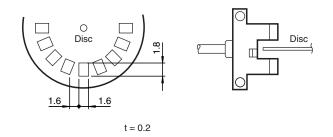
**Response frequency** The response frequency is the value when the disc is rotated, see figure.
