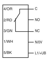
The relay-functions "NC" and "NO" bear on the switching mode "Light-ON". This complies to the default setting of the light/dark switch, located on top of the housing (factory setting).
