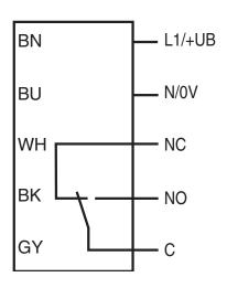
The relay-functions "NC" and "NO" bear on the switching mode "Light-ON".
