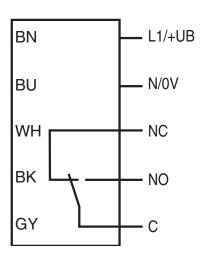
The relay-functions "NC" and "NO" bear on the switching mode "Dark-ON". This complies to the default setting of the light/dark switch (factory setting).
