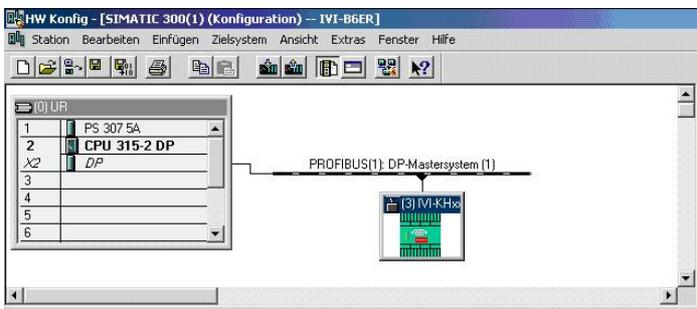
After that you have to determine the Profibus address. After double click on the symbol of the IVI a window will open. In this window you can configure the Profibus address.
