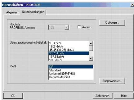
In the next step the Identification System IVI-KHD2-4HB6 have to connect to the ProfibusDP-Mastersystem. For this you must transfer “IVI-KHxx-4HB6” out of the Hardware index into the Master system.
