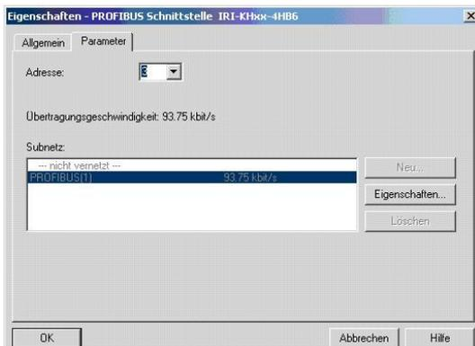
This address must be the same as on the top side of the unit adjusted address. After this you must define the addresses of the Input and Output of the IVI. By transfer of the address modules out of the Hardware index into the slots of the chart.
