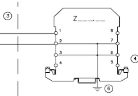
Any Simple Apparatus (2) or I.S. device with Entity Concept parameters (1) ( $V_{max}$ ,  $I_{max}$ ,  $C_L$ ,  $L_L$ ) appropriate for connection to associated apparatus with Entity Concept parameters listed below.
