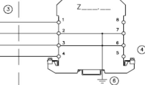
Any Simple Apparatus (2) or I.S. device with Entity Concept parameters (1) ( $V_{max}$ ,  $I_{max}$ ,  $C_L$ ,  $L_L$ ) appropriate for connection to associated apparatus with Entity Concept parameters listed below.
