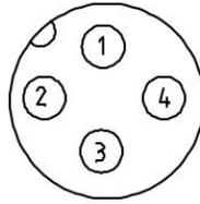
M12 (V1) connector pinout
