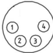
M8 (V31) connector pinout
