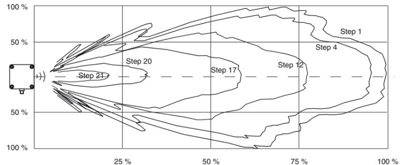
**Sensitivity adjustment for suppression of disturbing targets**
