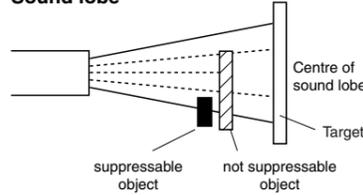
The suppression of the disturbing target is effected through reduction of the response sensitivity. This figure shows its effect on the response characteristics of the sensor. The sensor is preset on step 1 by the manufacturer.
