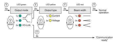
To change from IO-Link parameterization mode back to normal operation (analog signal on output), briefly disconnect the power supply from the
