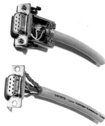
Advantage: metalised connector, shield clamped with the strain relief clamp
