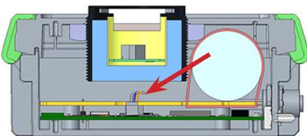
3. Plug the connection cable of the battery on the main board into one of the white connectors. Since the cables are internally connected, it does not matter which connector is used.
