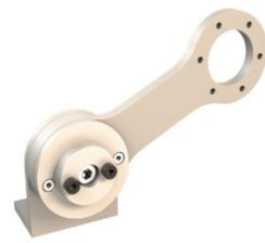
The spring arm MBT-36ALS120 is suitable for use of measuring wheels between 300mm and 500mm circumference on encoders with 58mm diameter. Due to the innovative 6 hole mounting a trouble-free cable routing is possible.
