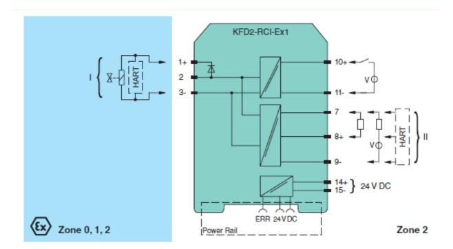
The KFD2-RCI-(EX)1 is a single channel Type A (HFT=0) device with low complexity and with a systematic capability of SIL 3.
