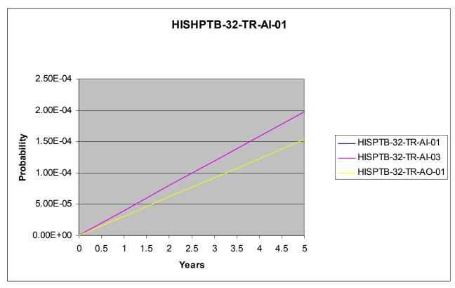
Figure 4: PFDavg vs. Proof Test Interval
