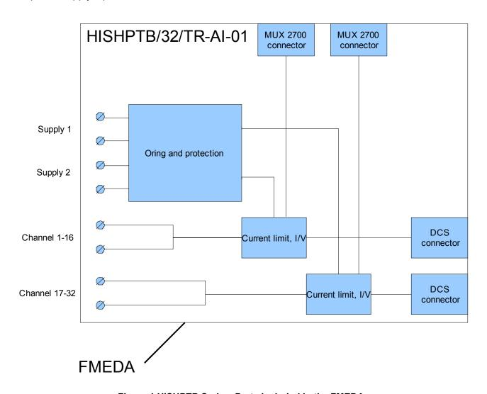
Figure 1 HISHPTB Series, Parts included in the FMEDA
