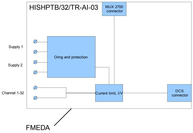
Figure 2 HISHPTB/32/TR-AI-03, Parts included in the FMEDA
