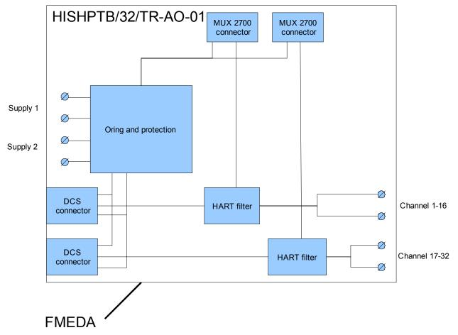
Figure 3 HISHPTB/32/TR-AO-01, Parts included in the FMEDA
