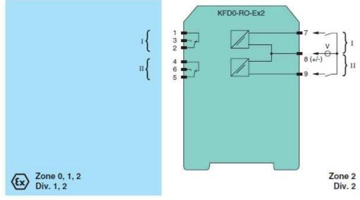
Fig. 1: Connection of the KFD0-RO-(Ex)2
