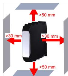
Derating ohne Einbauabstand // Derating without mounting distance // Derating sans distance de montage // Derating senza distanza di montaggio // Derating sin distancia de montaje
