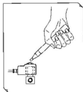
If the probe is placed near a magnetic field, for example of a solenoid valve, the LED indicator of the probe will light up.
