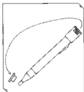
Using the test magnet, a self-test is performed.
