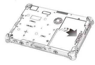
Slide the latch to the lock position to secure the battery.
