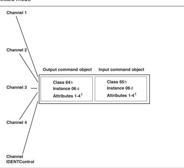
The five IDENT channels (four R/W heads, one configuration channel) are addressed using an input and an output instance, with the advantage that the controller requires less memory.
