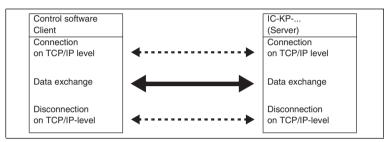
A connection must be established on the TCP/IP level before data can be exchanged. From this point onwards, commands can be sent from the client to the IC-KP-B12-V45 device.
