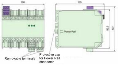
The following illustration applies in regard to the mechanical dimensions for products
