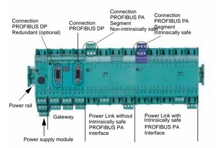
The gateway is used to convert the PROFIBUS DP protocol to the PROFIBUS PA protocol and back.
