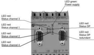
In normal operation, the LEDs should display the following state if there are no errors:
