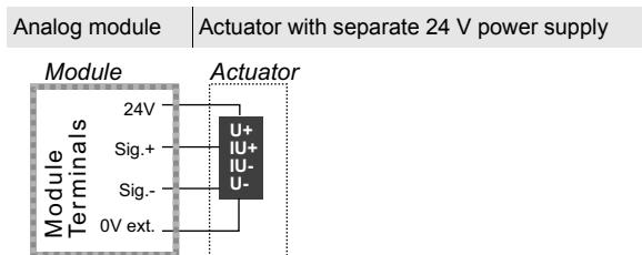
The separate 24 V are attached to terminals 3 (24 V) and 4 (0 V ext.), the analog signal to terminals 1 (I1 Sig.+) and 2 (I1 Sig.-) of channel 1. Corresponding channel 2 is attached via terminals 7 (24 V) and 8 (0 V ext.) as well as 5 (I2 Sig.+) and 6 (I2 Sig.-).
