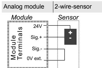
A 2-wire-sensor is attached to terminal 7 (24 V) and 8 (Sig.+) of channel 1. Terminals 9 (0 V ext.) and 10 (Sig.-) have to be connected to each other by using a bridge. Corresponding channel 2 is attached via terminal 1 (24 V) and 2 (Sig.+) as well as 3 (0 V ext.) and 4 (Sig.-).
