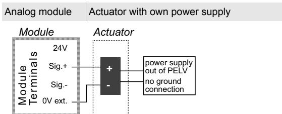
An actuator with own power supply (e. g. a voltmeter) is attached to terminals 8 (Sig.+) and 9 (0 V ext.) of channel 1, as well as terminals 2 (Sig.+) and 3 (0 V ext.) of channel 2.
