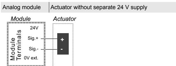
A 2-wire-actuator is attached to terminal 8 (Sig.+) and 10 (Sig.-) of channel 1. Corresponding channel 2 is attached via 2 (Sig.+) and 4 (Sig.-).
