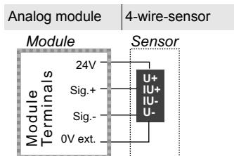
A 4-wire-sensor is attached to terminal 7 (24 V), 8 (Sig.+), 9 (0 V ext.) and 10 (Sig.-) of channel 1 see figure above for details. Corresponding channel 2 is attached via 1 (24 V) and 2 (Sig.+) as well as 3 (0 V ext.) and 4 (Sig.-).
