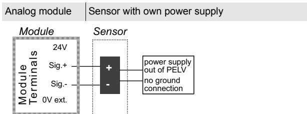
A sensor with own supply is attached for channel 1 to terminal 1 (I1 Sig.+) and 2 (I1 Sig.-) respectively for voltage input to terminals 9 (U1 Sig.+) and 10 (U1 Sig.-) of channel 1. Corresponding channel 2 is attached for current input via 5 (I2 Sig.+) and 6 (I2 Sig.-) respectively for voltage input via 11 (U2 Sig.+) and 12 (U2 Sig.-).
