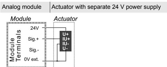
The separate 24 V are attached to terminal 7 (24 V) and 9 (0 V ext.), the analog signal to terminal 8 (Sig.+) and 9 (0 V ext.) of channel 1. Corresponding channel 2 is attached via terminals 1 (24 V) and 3 (0 V ext.) as well as 2 (Sig.+) and 3 (0 V ext.).
