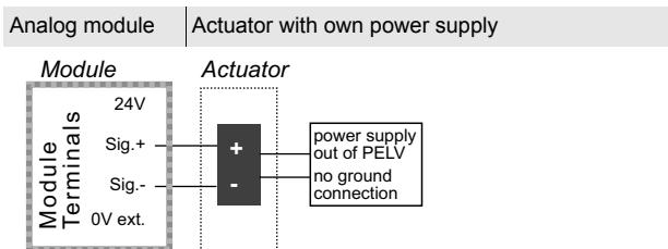
An actuator with own power supply (e. g. an ampmeter) is attached to terminal 1 (I1 Sig.+) and 2 (I1 Sig.-) of channel 1. Corresponding channel 2 is attached via 5 (I2 Sig.+) and 6 (I2 Sig.-).
