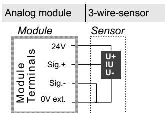
A 3-wire-sensor is attached to terminal 3 (24 V), 1 (I1 Sig.+) for current input respectively 9 (U1 Sig.+) for voltage input and 4 (0 V ext.) of channel 1. Terminals 4 (0 V ext.) and 2 (I1 Sig.-) for current input respectively 10 (U1 Sig.-) for voltage input have to be connected to each other by using a bridge.
