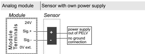
A sensor with own supply is attached to terminal 8 (Sig.+) and 10 (Sig.-) of channel 1. Corresponding channel 2 is attached via 2 (Sig.+) and 4 (Sig.-).
