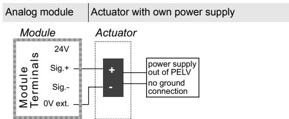
An actuator with own power supply (e. g. a voltmeter) is attached to terminals 9 (U2 Sig.+) and 4 (0 V ext.) of channel 1, as well as terminals 11 (U2 Sig.+) and 8 (0 V ext.) of channel 2.
