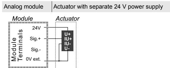
The separate 24 V are attached to terminal 3 (24 V) and 4 (0 V ext.), the analog signal to terminal 9 (U2 Sig.+) and 4 (0 V ext.) of channel 1. Corresponding channel 2 is attached via terminals 7 (24 V) and 8 (0 V ext.) as well as 11 (U2 Sig.+) and 8 (0 V ext.).
