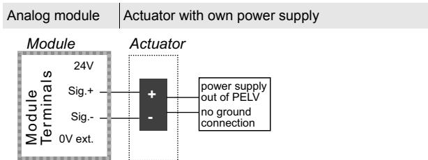
An actuator with own power supply (e. g. an ampmeter) is attached to terminal 8 (Sig.+) and 10 (Sig.-) of channel 1. Corresponding channel 2 is attached via 2 (Sig.+) and 4 (Sig.-).
