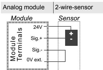
A 2-wire-sensor is attached to terminal 3 (24 V) and 1 (I1 Sig.+) of channel 1 for current input respectively to 9 (U1 Sig.+) for voltage input. The terminals 3 (0 V ext.) and 2 (I1 Sig.-) for current input respectively 10 (U1 Sig.-) for voltage input have to be connected to each other by using a bridge.
