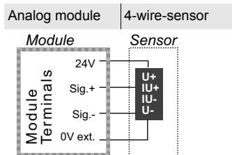
A 4-wire-sensor is attached to terminal 3 (24 V), 1 (I1 Sig.+) for current input respectively 9 (U1 Sig.+) for voltage input, 4 (0 V ext.) and 2 (I1 Sig.-) for current input respectively 10 (U1 Sig.-) of channel 1 see figure above for details.
