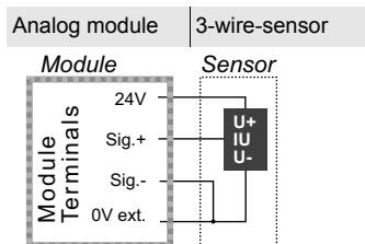
A 3-wire-sensor is attached to terminal 7 (24 V), 8 (Sig.+) and 9 (0 V ext.) of channel 1. Terminals 9 (0 V ext.) and 10 (Sig.-) have to be connected to each other by using a bridge. Corresponding channel 2 is attached via terminal 1 (24 V) and 2 (Sig.+) as well as 3 (0 V ext.) and 4 (Sig.-).
