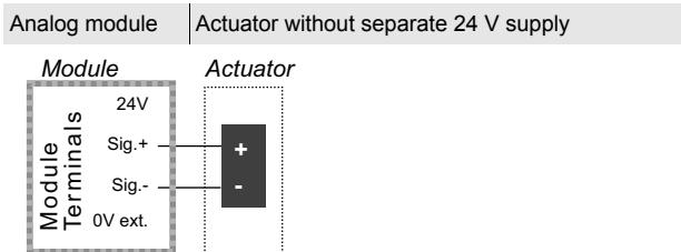
A 2-wire-actuator is attached to terminal 1 (I1 Sig.+) and 2 (I1 Sig.-) of channel 1. Corresponding channel 2 is attached via 5 (I2 Sig.+) and 6 (I2 Sig.-).
