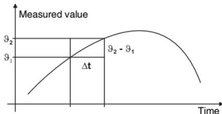
Select a sufficiently high value for  $\Delta t$  to ensure that temperature fluctuations relevant for your application which might occur during this time cannot cause any problem. This means that not only insignificant measured value fluctuations must be tolerated. Select a sufficiently low value for  $\Delta t$  to ensure that relevant minimum and maximum measured values are not hidden.
