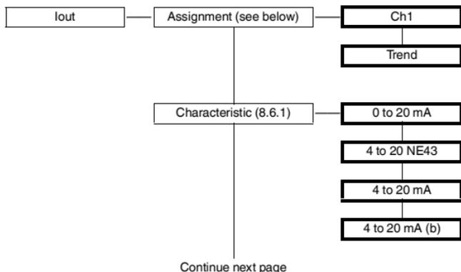
If you select the **assignment** *Ch1*, the output on the current output is proportional to the measured value of the device. This is the **normal** selection.
