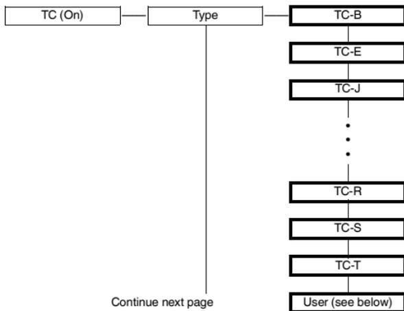
By means of the PACTware™ operating software, it is possible to enter an individual characteristic for a special thermocouple. Afterwards, you can select this characteristic via **User**.
