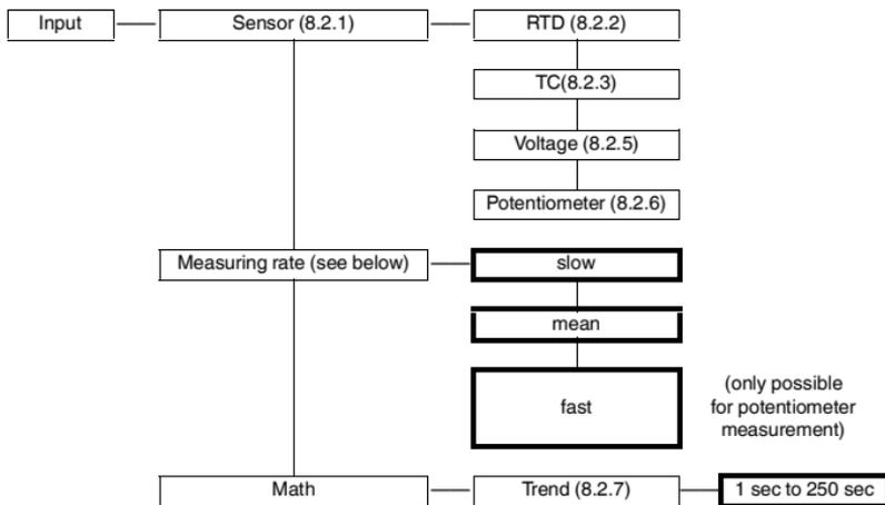
The precision values indicated in the data sheet refer to the **mean Measuring rate**. If the measuring rate is *fast*, the device measures more frequently, whereas the *slow* measuring rate delivers more precise results. The fast measuring rate is only possible for the potentiometer measurement.
