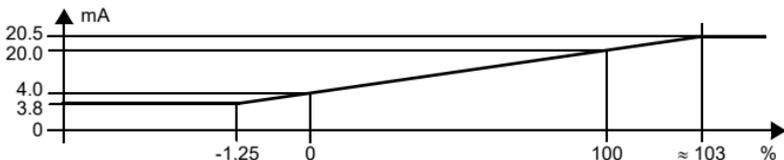
For this setting, the initial value is converted to 4 mA and the final value to 20 mA. Intermediate values are converted proportionally.
