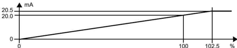
For this setting, the start value is converted to 0 mA and the final value to 20 mA. Intermediate values are converted proportionally.
