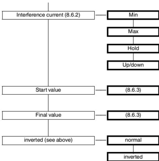
If you select the **inverted** characteristic, the representation of the start value and the final value is inverted (see section 8.6.1).
