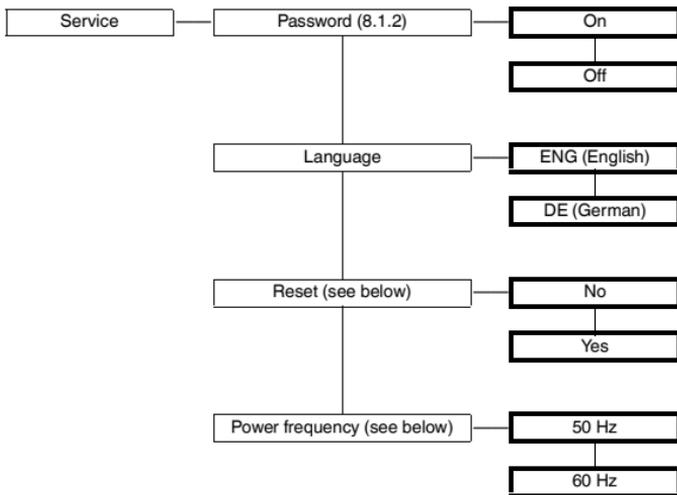
**Reset:** If Yes flashes and you press the OK key, the device settings are reset to the factory settings except for the sensor type (see section 8.8, for the selection of the sensor type see section 8.2.1). All inputs (except for the sensor type) which you have been performed in the parameterization mode at any time are lost.
