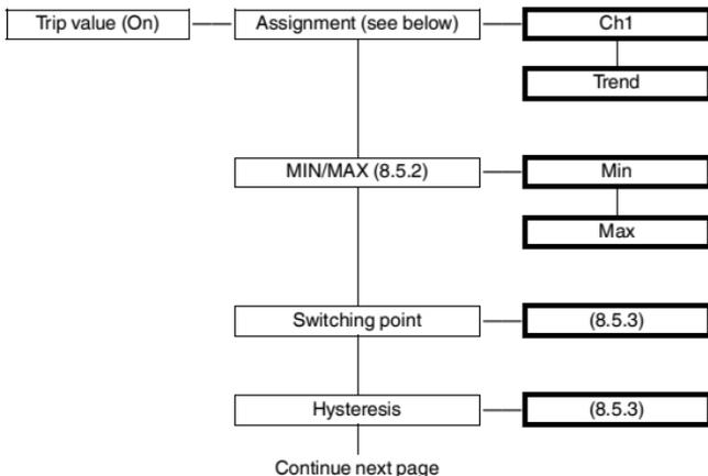
If you select the **assignment** *Ch1*, the limit monitoring refers to the measured value of the device. This is the **normal** selection.
