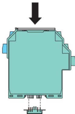
The devices of the Pepperl+Fuchs K systems and also the temperature converters can be fitted to a 35 mm DIN rail according to EN 60715. Simply snap the devices **vertically**; avoid tilting/sloping.
