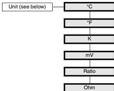
The **unit** is used for measured-value display and for all corresponding settings in the parameterization mode. The selection of the sensor type determines which units are available (see section 8.2.1). In some cases, the selected measuring type is also relevant (see section 8.2.6):
