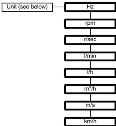
The **Unit** is used for display of measured values and for all corresponding settings in parameter is at ion mode. The device always works internally in Hz (actually in mHz = 0.001 Hz).
