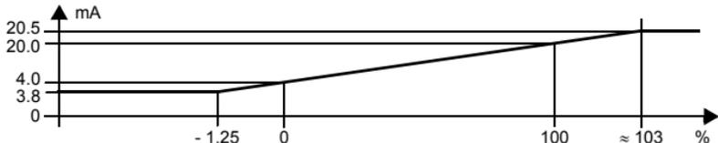
For this setting, the initial value is converted to 4 mA and the final value to 20 mA. Intermediate values are converted proportional.
