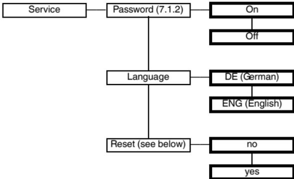
**Reset:** If the value *yes* is shown flashing and you press the OK key, all parameters in the device will be reset to their factory settings. All entries you have ever made in parameterization mode will be lost.
