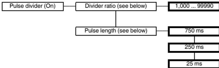
The number of input pulses is divided by the **divider ratio** and switched to the output. The relays can only be used in certain cases as signal divider outputs due to the maximum switching frequency < 2 Hz.
