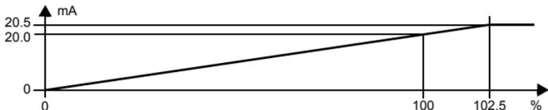
For this setting, the start value is converted to 0 mA and the final value to 20 mA. Intermediate values are converted proportional.
