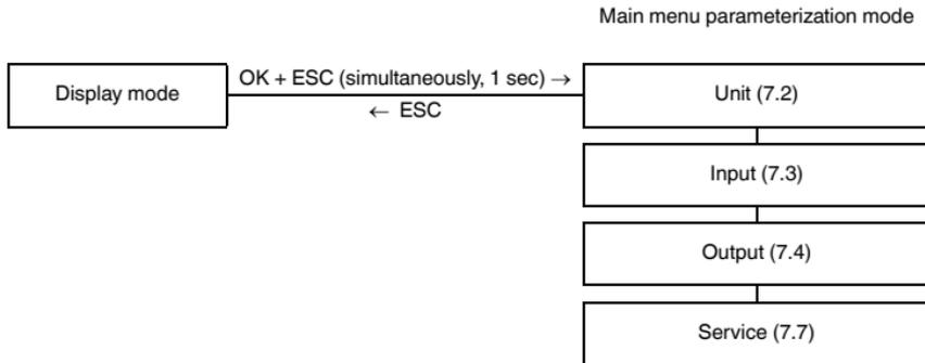
You can return to display mode from any point in the menu in parameterization mode by pressing the ESC key (possibly multiple times). If you do not press any key for 10 minutes in parameterization mode, the device automatically switches back into display mode.
