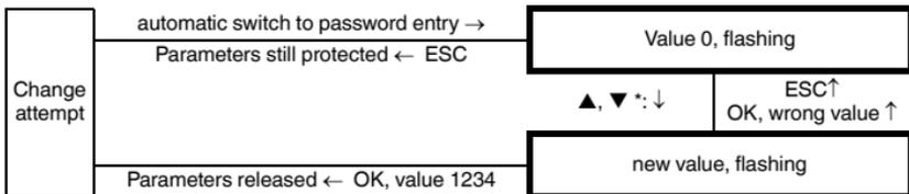
\*If the ▲ or ▼ keys are pressed, the value changes stepwise; if the ▲ or ▼ keys are held down for a longer period, the value "rolls" to higher or lower values.
