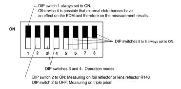
The lens reflector R140 does not represent a triple prism!
