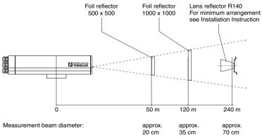
Figure 5.4 Reflector arrangement (EDM side view)
