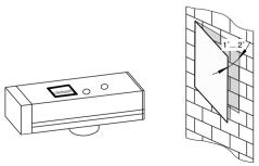
Figure 5.7 3-D view of the relationship between sensor orientation and reflector tilt angle orientation
