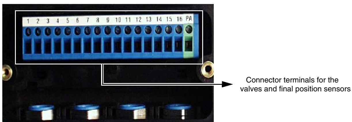
Figure 3.4: Location and designation of the connector terminals for the valve connection including final position feedback contacts
