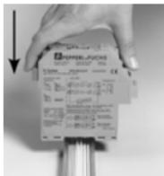
The devices of the K-System from Pepperl+Fuchs can be mounted on a 35 mm top-hat rail corresponding to EN 60715. The devices must be snapped onto the rail **vertically**, and never slanted or tipped to the side.
