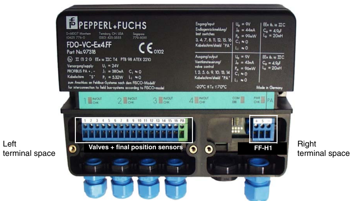
Figure 3.2: Valve Coupler with the terminal space covers removed
