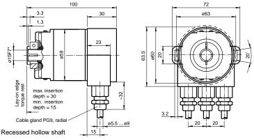
\* shaft can be reduced to ø10F7 or ø12F7 by using an adapter
