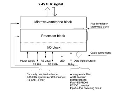
Bild 4.3: Communicator architecture
