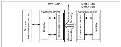
Bild 4.2: Communicator function within the overall system
