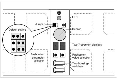
Bild 7.1: Control panel's location
