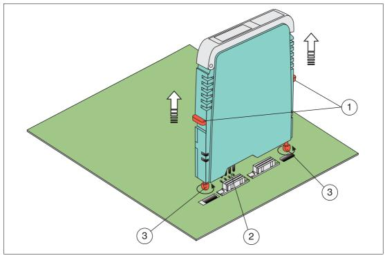
Figure 8.1 Dismounting of an H-System isolated barrier
