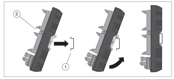
Figure 4.2 Termination board mounting
