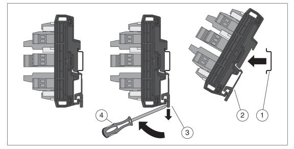
Figure 8.4 Termination board dismounting
