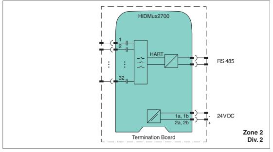
Figure 4.7 Connection of the HiDMux2700 HART multiplexer master
