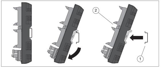
Figure 8.3 Termination board dismounting
