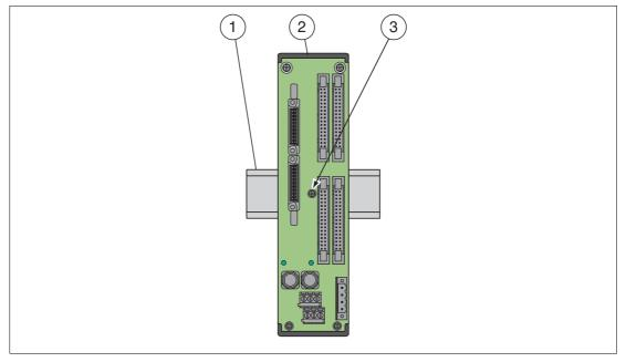
Figure 4.3 Termination board fixing
