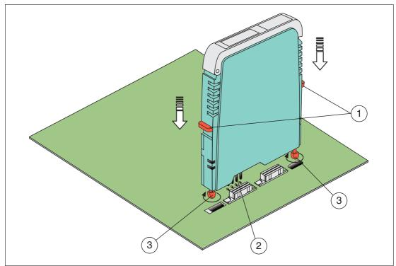
Figure 4.6 Mounting of an H-System isolated barrier
