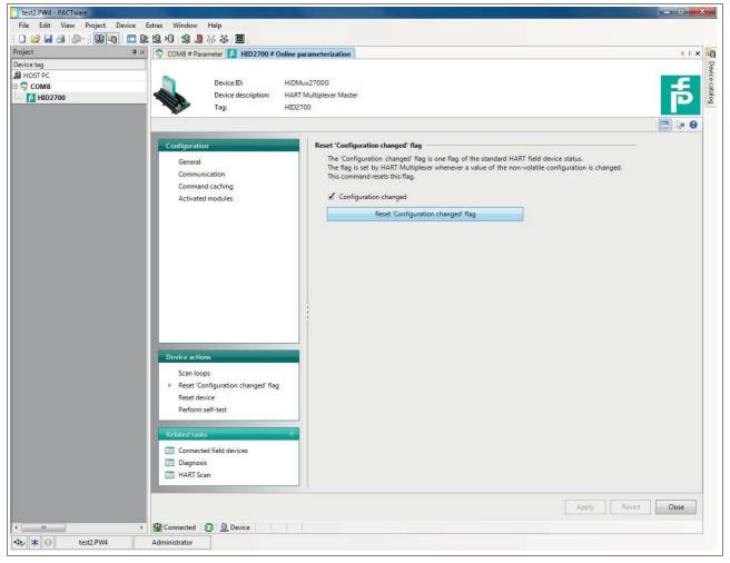
Figure 7.5 Reset "Configuration changed" flag window
