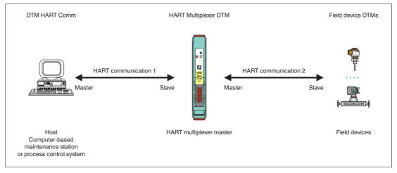
Figure 6.1 Software components
