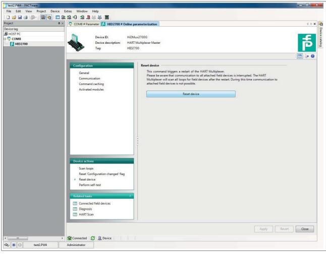
Figure 7.6 Reset device window
