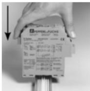
The devices of the K-system from Pepperl+Fuchs and thus also the Timer Relay KF\*\*-DU-Ex1.D can be mounted on a 35 mm standard rail corresponding to DIN EN 60175. The devices must be snapped onto the rail **vertically**, and never slanted or tipped to the side.
