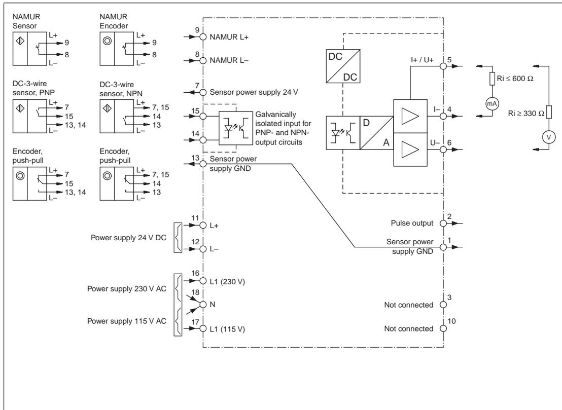
Figure 5.1 Connection diagram
