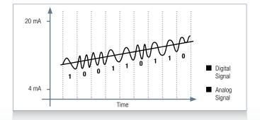
level on top of the 4...20 mA control signal. This enables two-way field communication to take place and makes it possible for additional information beyond the normal process variable to be communicated to/from a smart field instrument.
