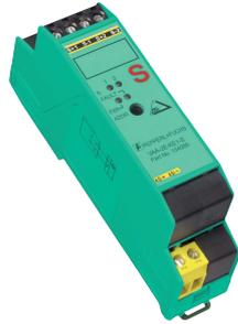
The VAA-2E-KE1 is an AS-Interface safety module with two safety-related inputs. A dual-channel mechanical switch or single-channel mechanical switch can be connected to the two inputs. The housing is only 22.5 mm wide and 48.5 mm tall and takes up little space in the switch cabinet. A snap-on function mounts the module onto the 35 mm mounting strip in line with EN 50022. An addressing socket is integrated in the module.
