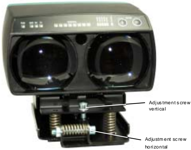
Figure 6.2 mounted LS610 with adjustment elements
