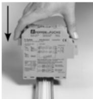
The devices of the K-systems from Pepperl+Fuchs and thus also the temperature converters KFD2-UT2-(Ex)\*(-1) can be mounted on a 35 mm top-hat rail corresponding to DIN EN 50022. The devices must be snapped onto the rail **vertically**, and never slanted or tipped to the side.
