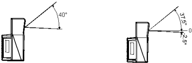
Figure 5.3 Maximum deflection and asymmetry of the oscillating mirror
