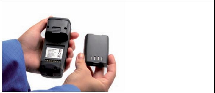
2. Slide the plastic tab on the battery into the corresponding recess on the Handheld.
