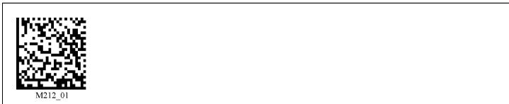
2. To activate 2D windowing for a reading area of 512 x 512 pixels, scan the code **Medium 2D Codes (512 x 512 pixels)**:
