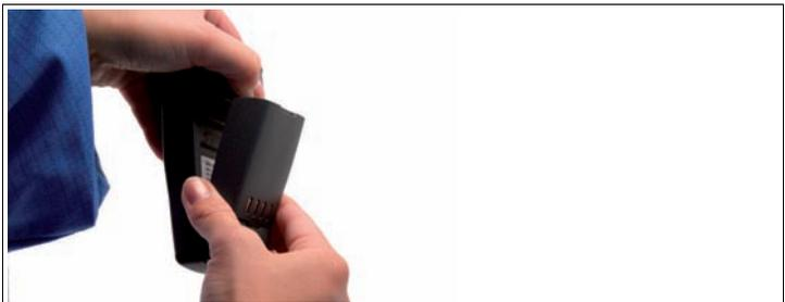
3. Push the locking device upwards and push in the battery.
