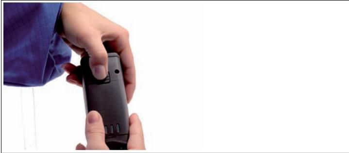
4. Push the battery in the Handheld, hold in position and release the locking device so that the battery engages.
