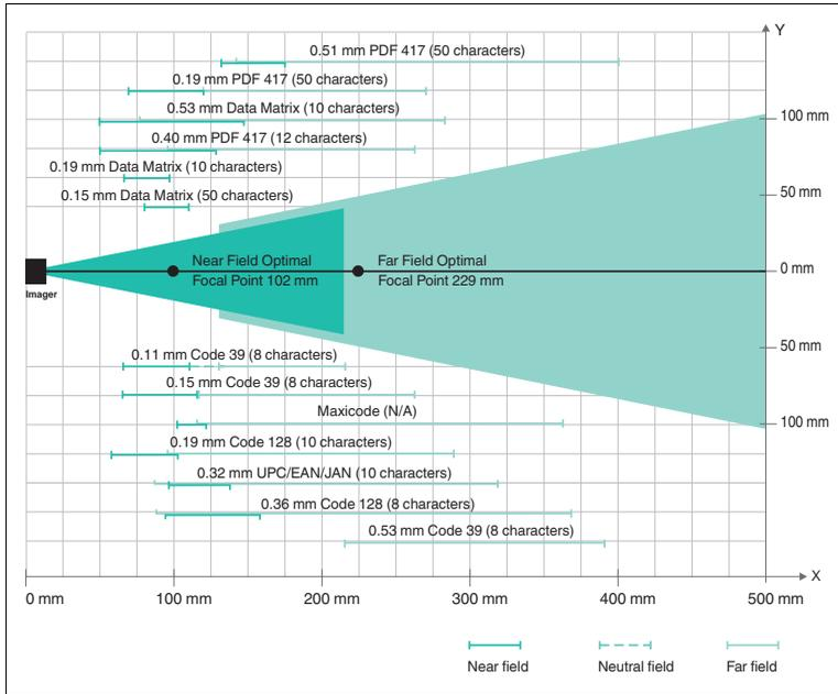
Figure 4.2: Field of vision of handheld ODT-HH-MAH200
